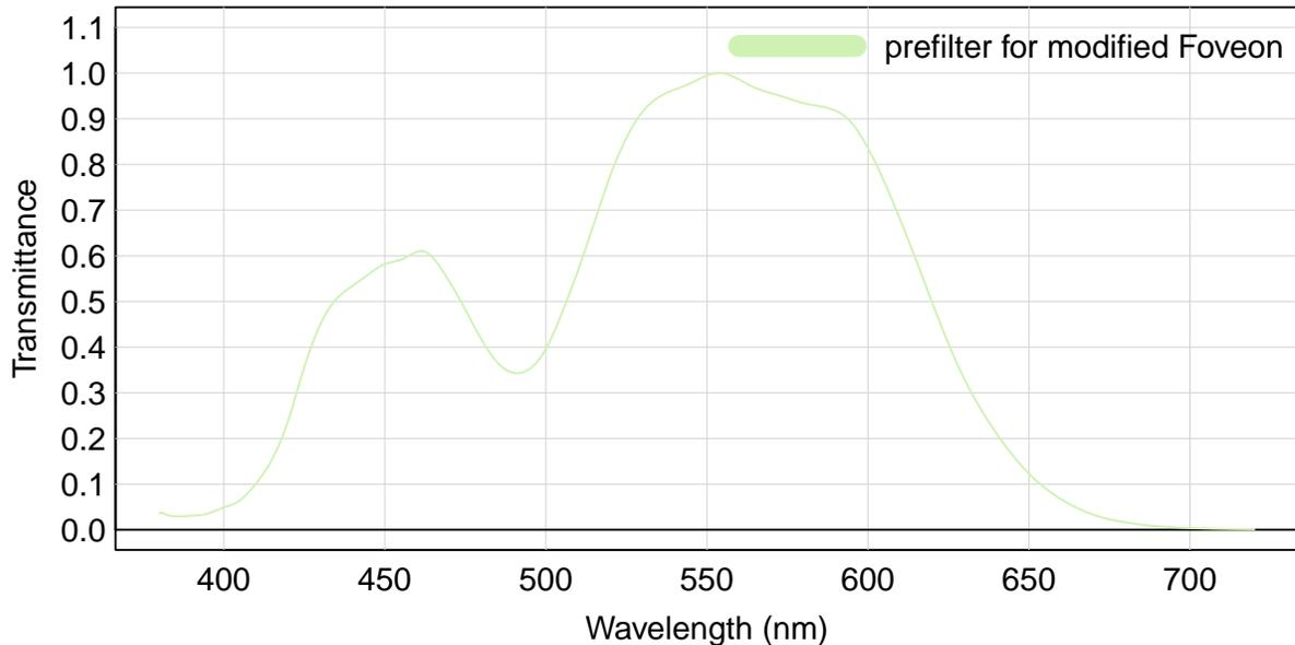
Figure 5: Prefilter for the modified Foveon camera
