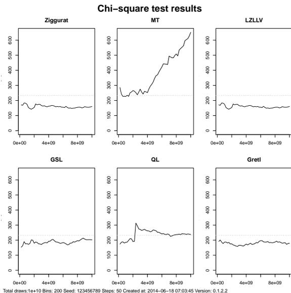
Fig. 6.  $\chi^2$  Test applied to Ziggurat generators
